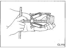
Remove release bearing using a suitable puller.
