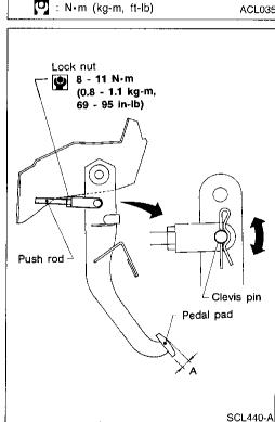
Adjust pedal free play by turning master cylinder push rod. Then tighten lock nut.
