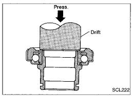
Install release bearing using a suitable drift.
